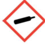
This pictogram means 'Contains gas under pressure'
